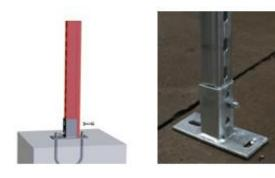
Install base bracket with expansion bolts or U-bolt to fix. And then fix post by 2 inner-hexagon socket bolts M10\*30 kits (contain 2 flats, 1spring, 1nut).
