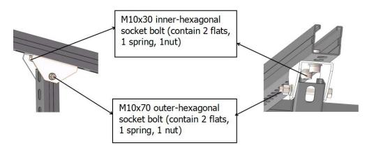
Hinge connected to post as the up image:
