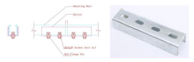
Rail splice is outside of the ends of the rails. We will use M10x30 inner-hexagonal socket bolt (contain 2 flats, 1spring, 1nut) to connect the rail splice and the rails
