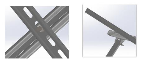
Use M10 square nut as nut to connect main beam and rail.
